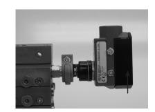
AC498-1 w/4 pin micro connector M12 X 1 & LED light. Couples to any M2500G metering valve. Rated to 5000 PSI (350 BAR). Requires 10-36 VDC. To be used with the SC400 Controller or customer PLC only. (See M12 Connectors below)
