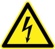
Safety symbol according to DIN 4844, warning about dangerous electric voltage.
