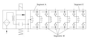
01 is equal to 0.1 cm<sup>3</sup> per piston stroke
