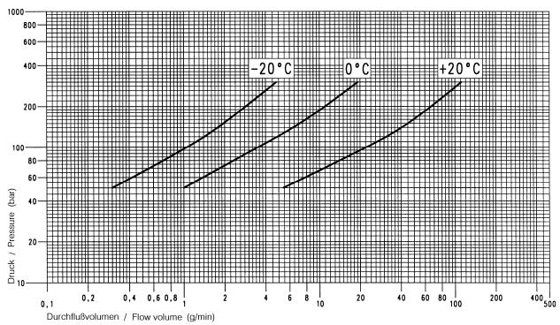
Flow medium: Grease Renolit MP Company: Fuchs Worked penetration NLGI-class 2
