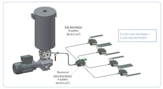
In the above example four equal sub-distributors are connected to a main distributor. The main distributor divides the quantity supplied by the pump into four equal parts. The lubrication points thus all receive the same quantity.
