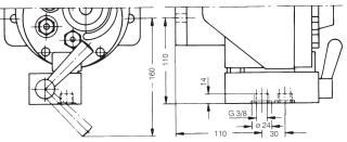
Pump with 4/2-way valve fitted for dual-line units
