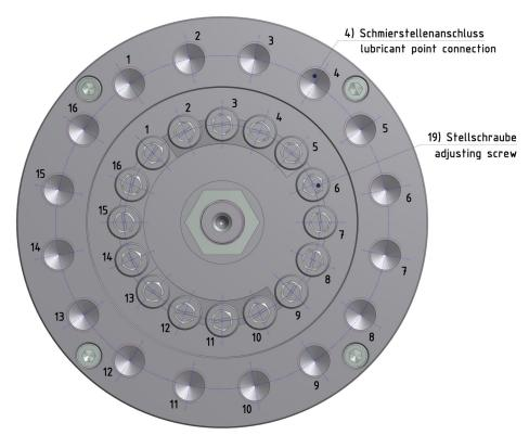
Assignment of delivery pistons to the feed-line connections.
